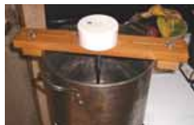
Homemade automatic pot stirrer is powered by a 120-volt electric motor that clamps to top of cooking pot. Motor shaft-drives an 8-in. long twisted metal paddle.
