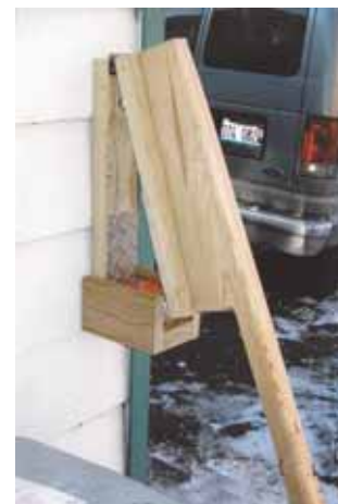
Operator pushes down on hinged handle to crush can against diamond steel plate.
