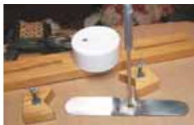
Homemade automatic pot stirrer is powered by a 120-volt electric motor that clamps to top of cooking pot. Motor shaft-drives an 8-in. long twisted metal paddle.
